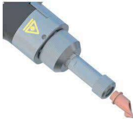
Figure 6-1 Schematic Diagram of Nozzle Tip Replacement
