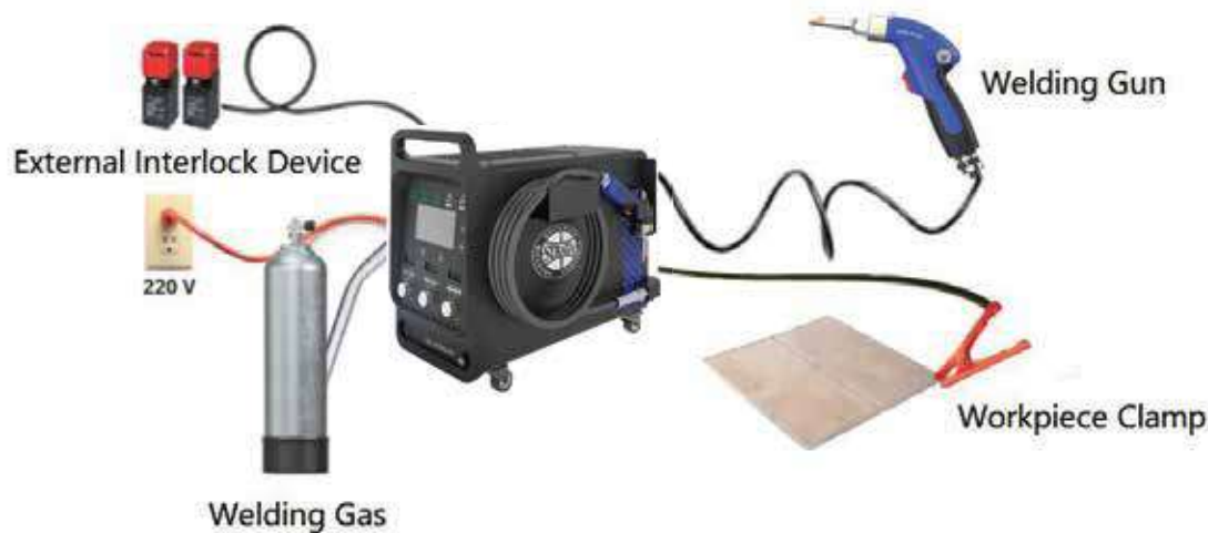
Figure 4-1 Typical Setup of the Welding System
